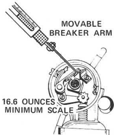
CHECK SIDE PLAY OF DISTRIBUTOR SHAFT
